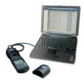
Data Transfer Adapter converts infrared signals from the instrument to standard RS-232 protocol. The adapter fits over the instrument in place of the cap and connects directly to a printer or computer.
